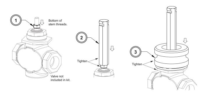
After the AV-811 adapter is installed, install the selected actuator and linkage (if required) according to the actuator installation instructions.
